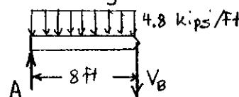
$$\begin{aligned} \textcircled{D} \sum M_A &= 0 \\ (4.8)(8)(4) - 8A &= 0 \\ A &= 19.2 \text{ kips} \\ \textcircled{D} \sum M_A &= 0 \\ -(4.8)(8)(4) - 8V_B &= 0 \\ V_B &= -19.2 \text{ kips} \end{aligned}$$
