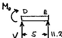
$$\begin{aligned} \textcircled{D} \sum M_D &= 0 \\ -M_D + (11.2)(5) &= 0 \\ M_D &= 56 \text{ kip-ft.} \end{aligned}$$
