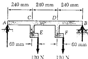
**5.44 and 5.45** Draw the shear and bending-moment diagrams for the beam and loading shown, and determine the maximum absolute value (a) of the shear, (b) of the bending moment.
