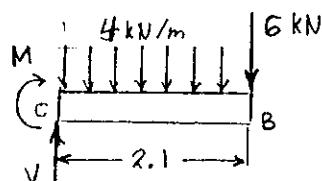
$$\text{For } W 310 \times 32.7 \quad S = 415 \times 10^3 \text{ mm}^3 = 415 \times 10^{-6} \text{ m}^3$$
