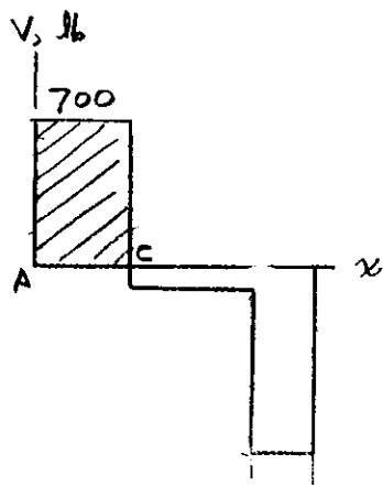
Shear curve from A to C:  $V = 700 \text{ lb.}$
