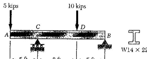
$$\text{Reaction at } C \quad \sum M_B = 0 \\ (18)(5) - 13C + (5)(10) = 0 \\ C = 10.769 \text{ kips}$$
