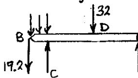
$$\begin{aligned} \textcircled{D} \sum M_E &= 0 \\ (19.2)(12) + (4.8)(2)(11) &= 0 \\ -10C + (32)(5) &= 0 \\ C &= 49.2 \text{ kips} \\ \textcircled{D} \sum M_C &= 0 \\ (19.2)(2) + (4.8)(2)(1) &= 0 \\ -(32)(5) + 10E &= 0 \\ E &= 11.2 \text{ kips} \end{aligned}$$
