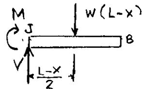
Replace distributed load by equivalent concentrated load.
