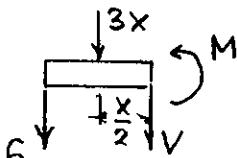
$$\text{At } C: \sum F_y = 0 \quad -6 - 3x - V = 0 \quad V = -6 - 3x \text{ kips.}$$
