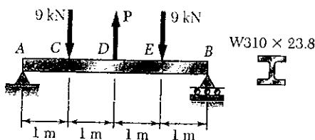
By symmetry the reactions at  $A$  and  $B$  are equal.
