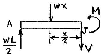
Replace distributed load by equivalent concentrated load.
