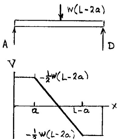
Calculate reactions after replacing distributed load by an equivalent concentrated load.
