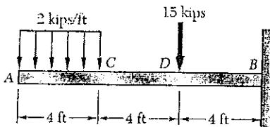
5.9 and 5.10 Draw the shear and bending-moment diagrams for the beam and loading shown, and determine the maximum absolute value (a) of the shear, (b) of the bending moment.
